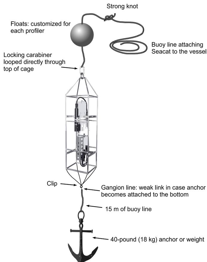
**Figure 4. Schematic diagram illustrating the water column profiler configuration used for deployment from IPHC setline survey vessels.**
