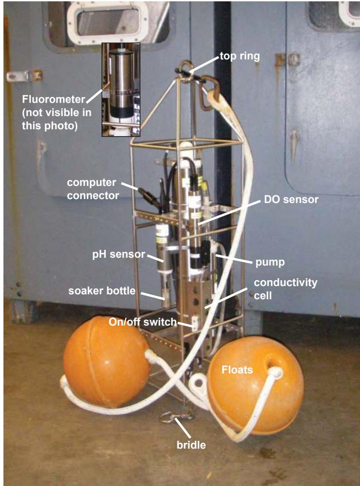
**Figure 5. Sea-Bird water column profiler used by the IPHC during the annual setline survey.**
