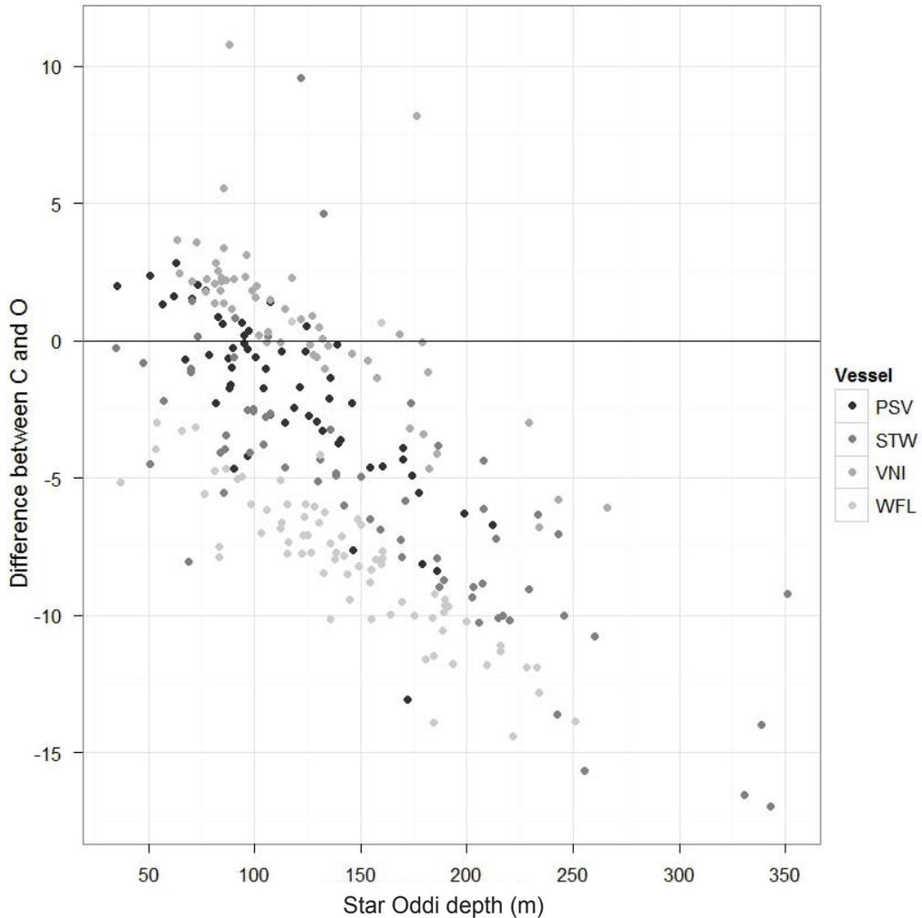
**Figure 10. The difference between the vessel depth-finding instruments and what was recorded by the Star Oddi (O-C). This shows that at shallow depths, the measurements were similar, but at deeper depths, the vessel instruments tended to overestimate the bottom depth.**
