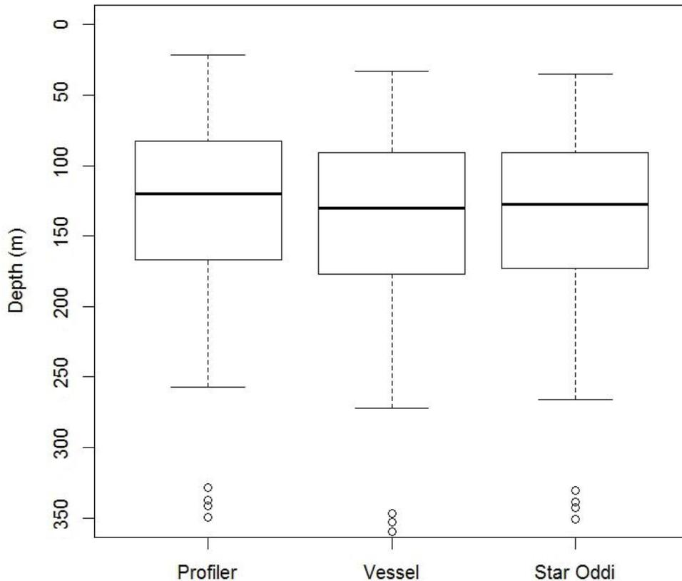
**Figure 7. Boxplot of the three datasets used in this analysis: maximum profiler depth, bottom depth as measured by vessel depth-finding instruments, and bottom depth as measured by Star Oddi sensors.**
