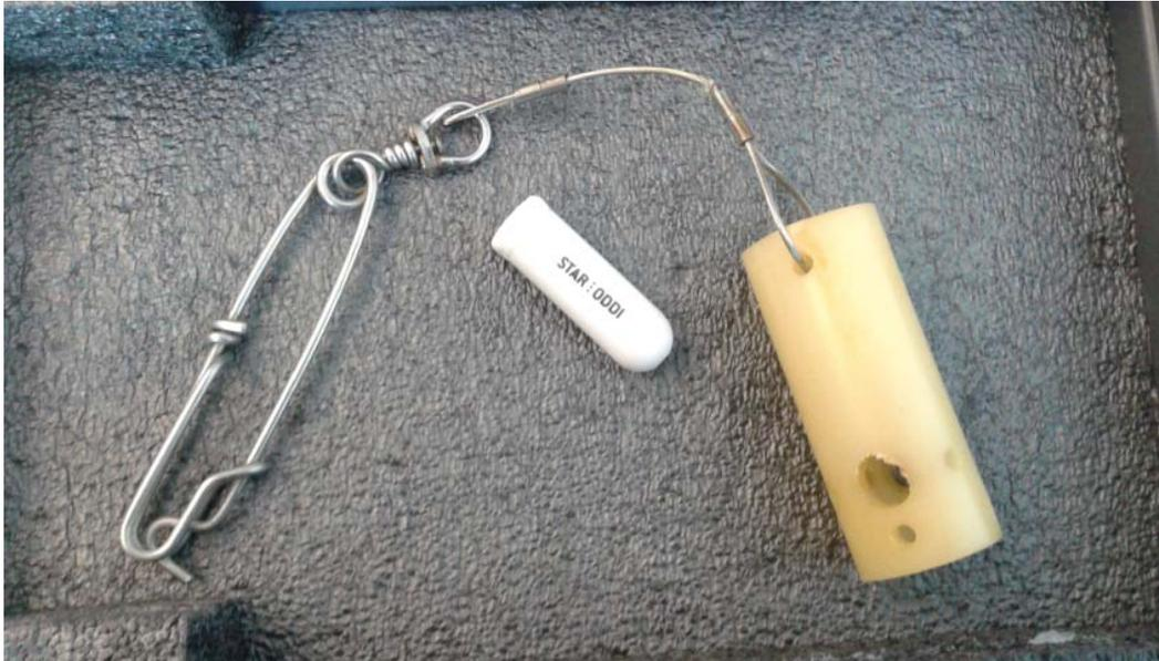
**Figure 6. Star-Oddi sensor and housing used in 2012 to reconcile the deepest profiler depth with bottom depth.**
