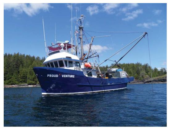
Seine-type vessel, *F/V Proud Venture*. Note pilothouse forward compared with a schooner type vessel where pilothouse is aft. Photo by Levy Boitor.
