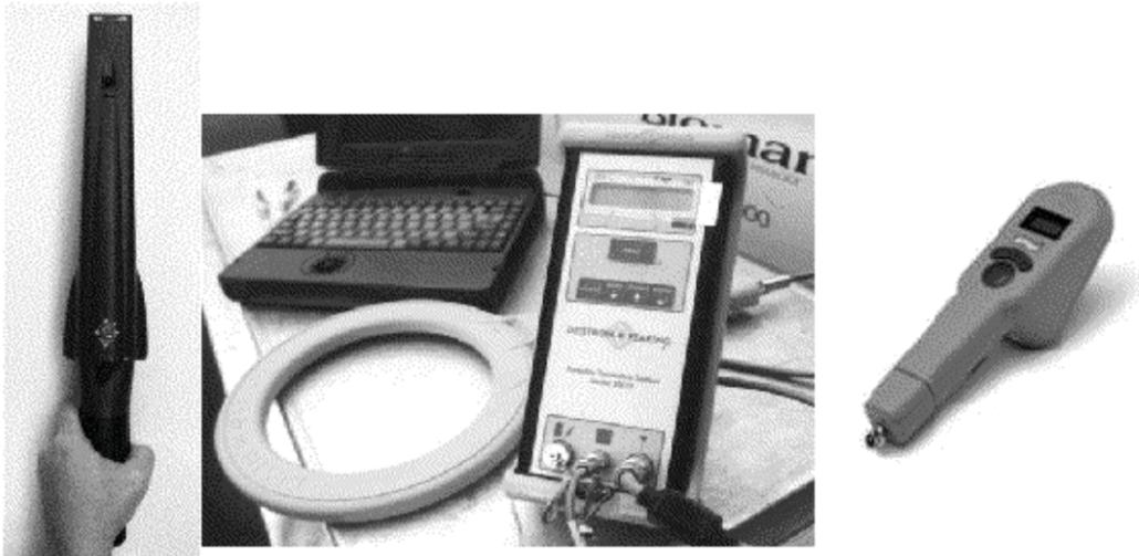
**Figure 3. Portable PIT tag readers (left to right): Coded Wire Tag detector; Destron-Fearing antenna and transceiver (“Destron reader”); Allflex boulder reader.**
