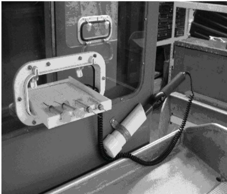
**Figure 6. IPHC data recording shack, showing needle tray, measuring cradle, and stick reader in holder.**
