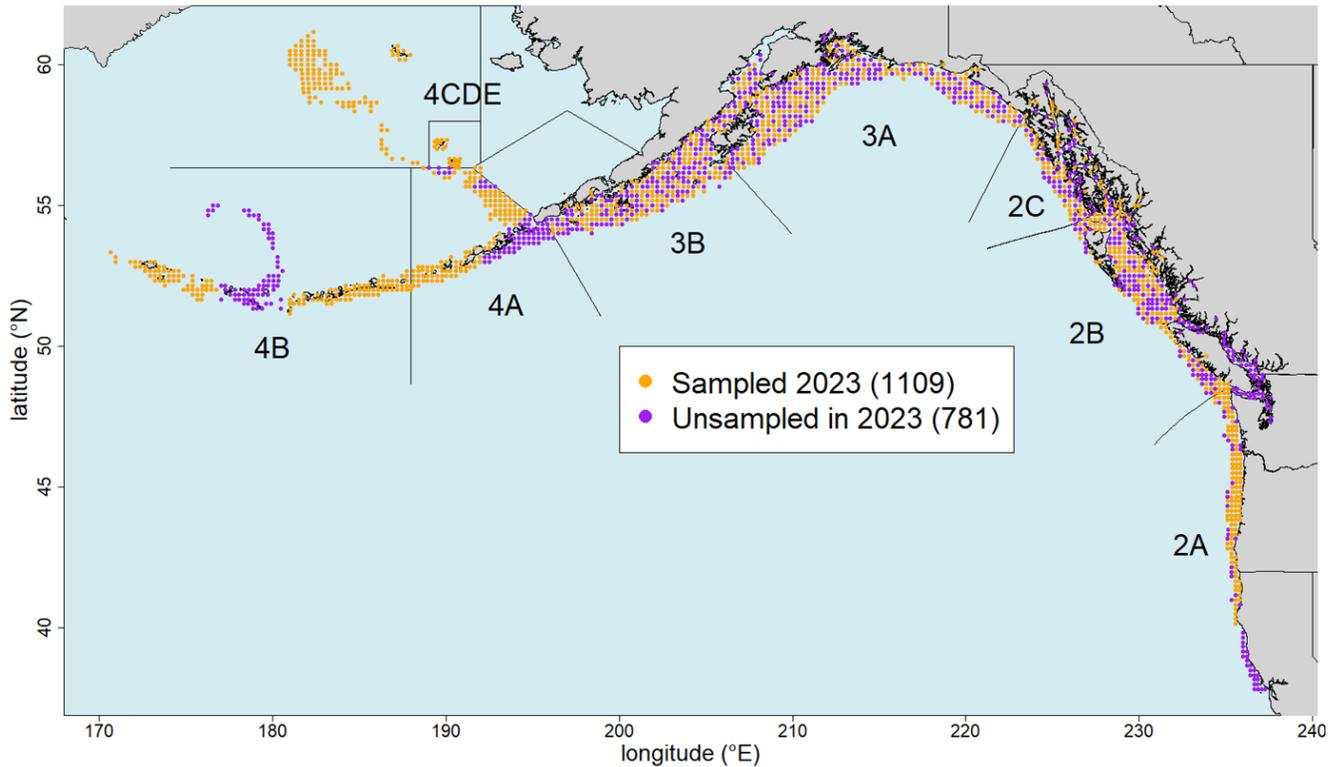
**Figure 2.** Proposed FISS design (pre-optimisation) in 2023 (orange circles) based on randomised sampling in 2B-3B, and a subarea design elsewhere. Purple circles are optional for meeting data quality criteria.
