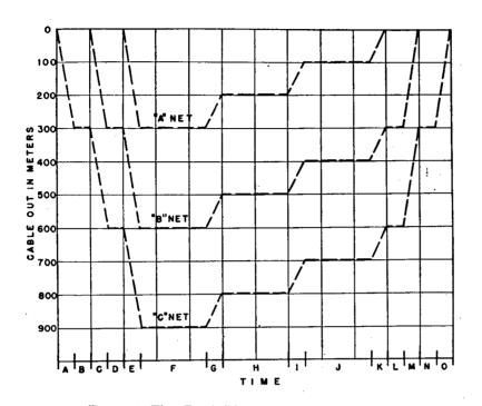
FIGURE 4. Time-Depth Diagram of a Standard Haul.
