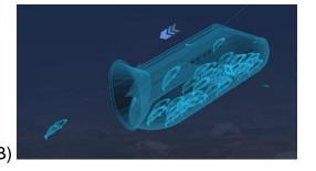
**Figure 1.** Schematic of underwater shuttle device, as it slides down the groundline (A) and cross-sectional view of fish released and contained within the device (B) (images from Sago Solutions presentation).
