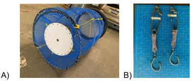
**Figure 4**. Shroud showing end cap and openings (A), and variable strength snaps attached to hooks by shortened stiff gangions (B).
