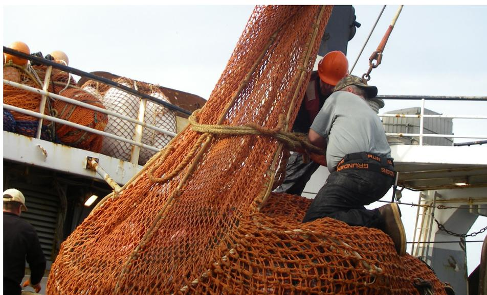
Bringing the codend aboard a trawl vessel (Photo taken during the NOAA groundfish trawl survey). Photo by Ben Burnett.
