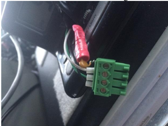
Figure 13. (a) Image of AMR leads from Hydro sensor 13 (b) NOAA hydro switch sensor installed
