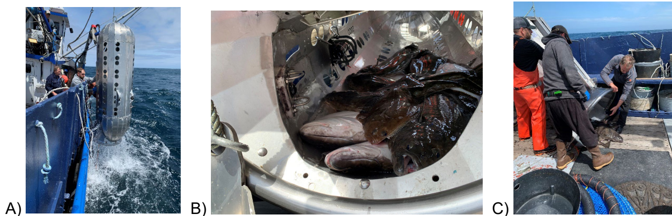
Figure 7. Shuttle being retrieved A), catch entrained in shuttle B), and catch being emptied onto the vessel deck.
