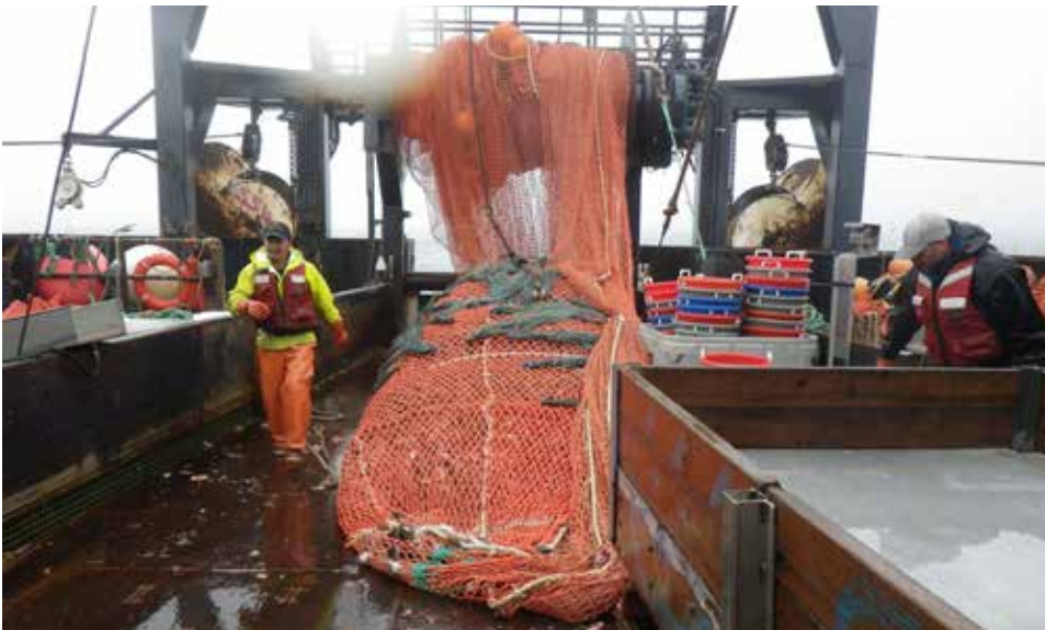
Incidental catch of Pacific halibut can occur with any gear including trawl, longline, and pot. Pictured here is a trawl codend which has just been pulled aboard the survey vessel. Photo by Paul Logan.
