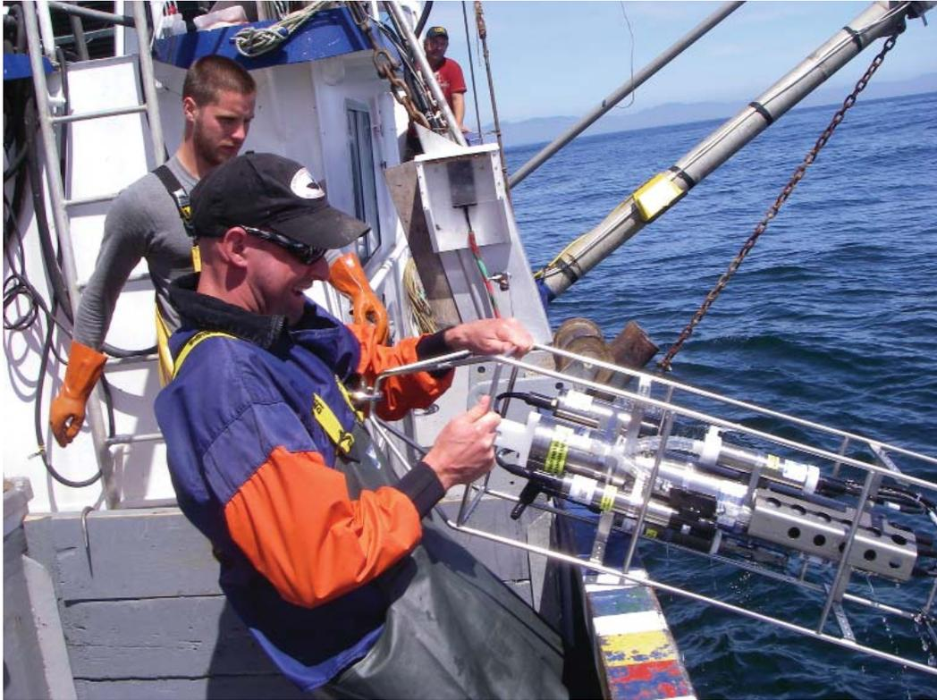
**A water column profiler is deployed at each setline survey station to collect environmental data on the halibut grounds. Photo by Beth Dubofsky.**
