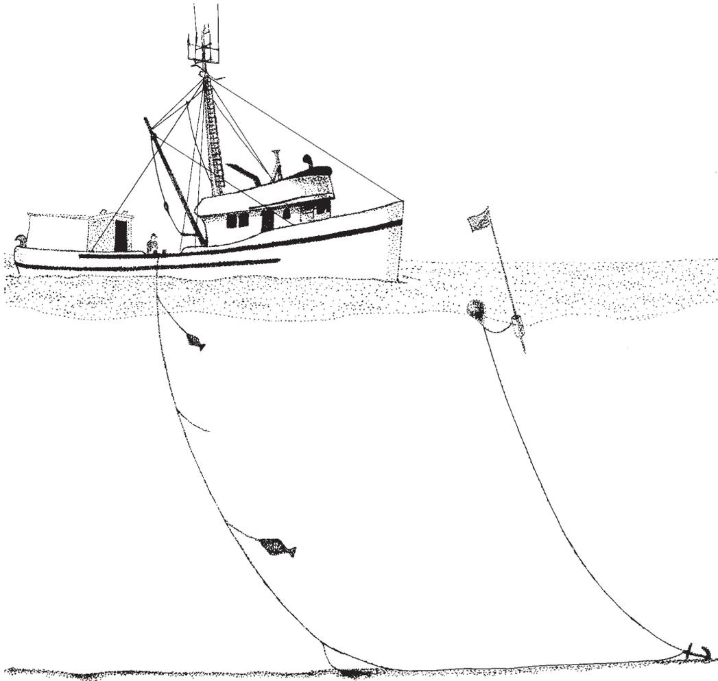
**Figure 8. Halibut fishing gear.**
