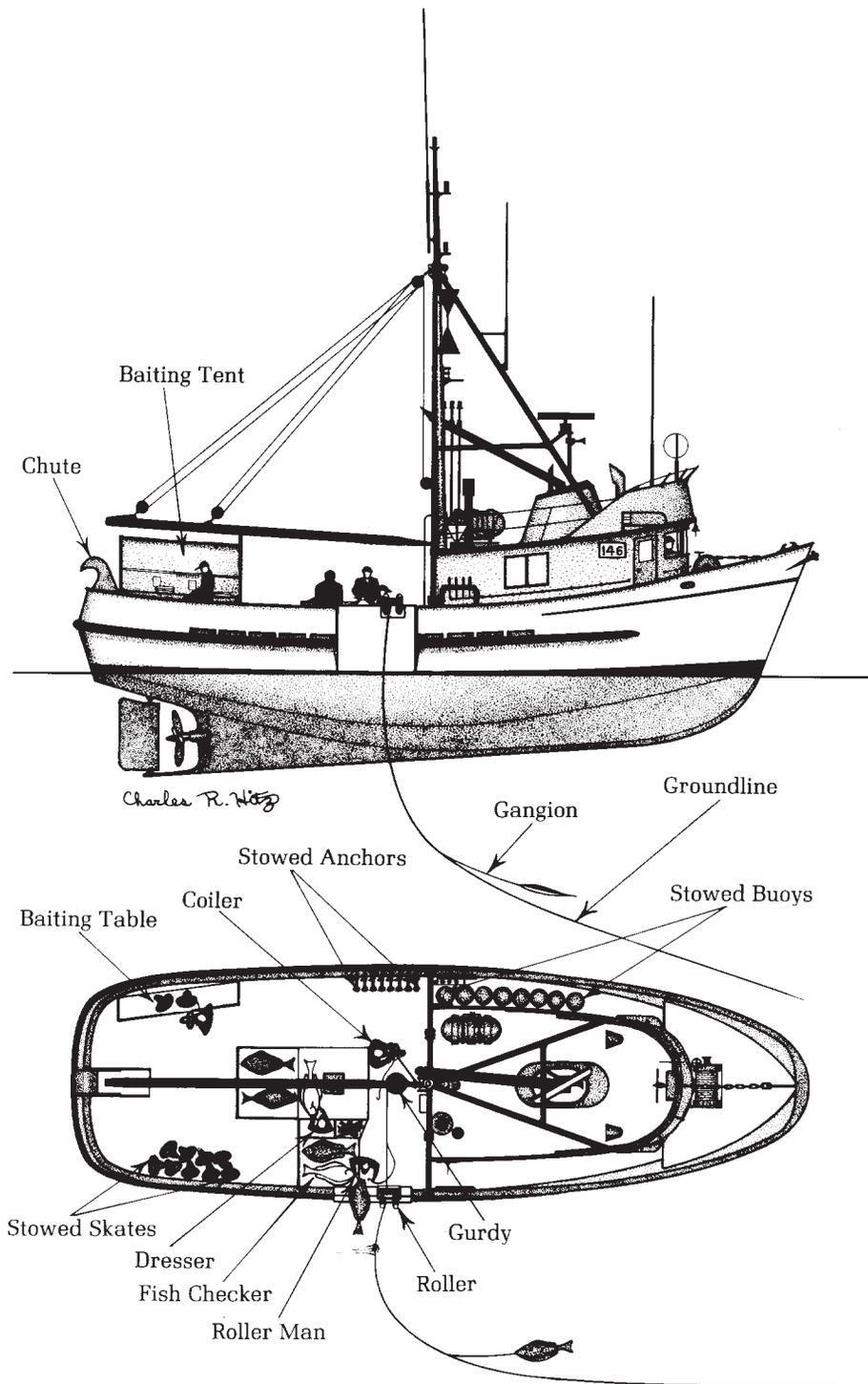
Figure 9. Deck layout of a vessel fishing with conventional gear.
