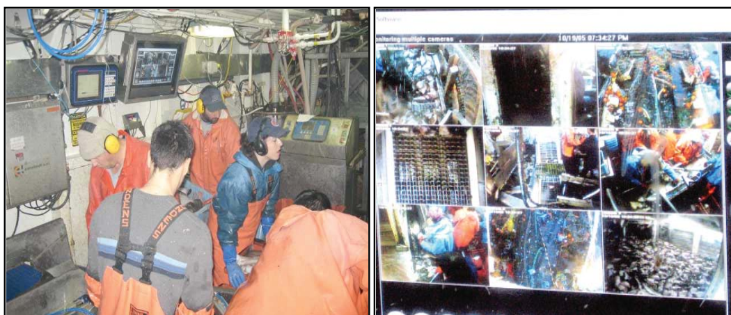
Figure 4. LCD screen available to crew in sorting area (left) and close up photograph of the LCD screen showing nine camera views simultaneously (right).
