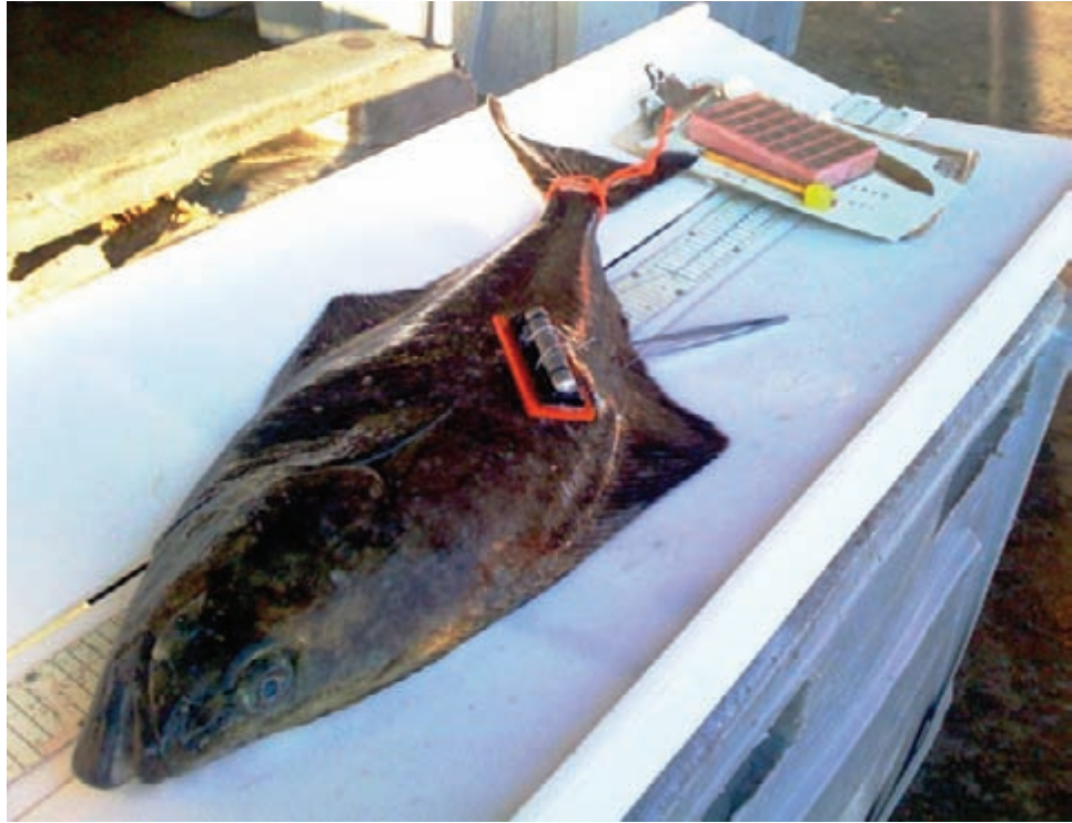
This halibut has been fitted with an external archival tag. Photo by Tim Loher.
