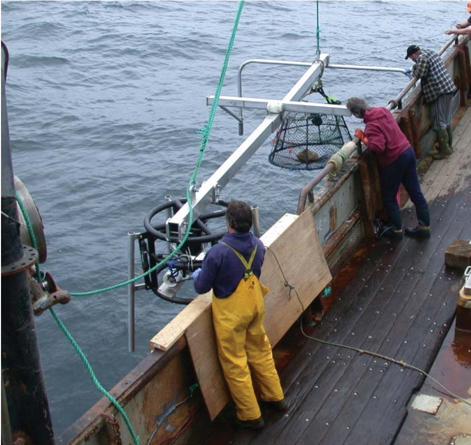
Launching the DIDSON from the deck of the F/V Ocean Pearl . Photo by Steve Wischniowski.
