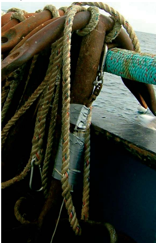
The WaDar is used on surveys and in the Pribilof Islands to monitor bottom temperature. The device is attached to an anchor and thrown over with the gear. IPHC photo archive.
