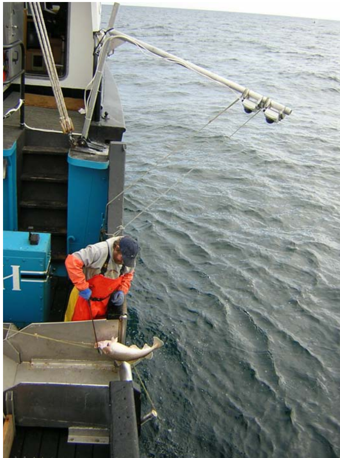
Video cameras are mounted above the roller to monitor the catch. Photo by Robert Ames.
