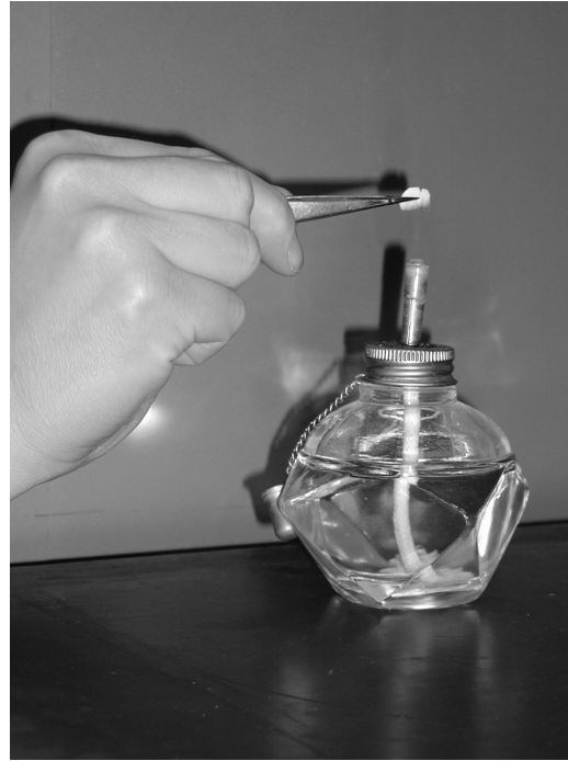
Figure 17. Burning a halibut otolith section over an alcohol flame.
