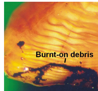
Figure 71. Enlargement of the burnt section in Figure 68 showing burnt-on debris.
