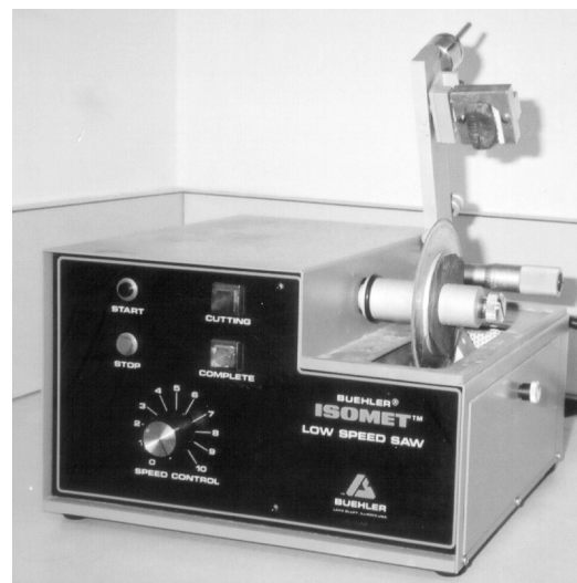
Figure 16. Low speed Isomet saw used for cutting otoliths.
