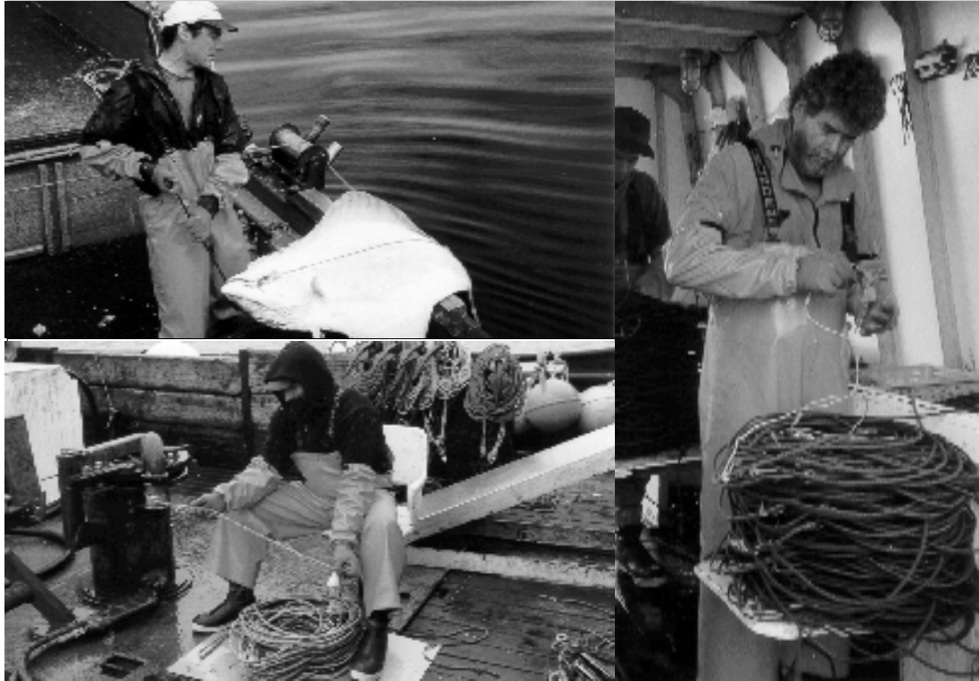
Top left: hauling in a halibut. Bottom left: Coiling a skate of gear as it's hauled in by a power gurdy. Right: Baiting a skate of gear.
