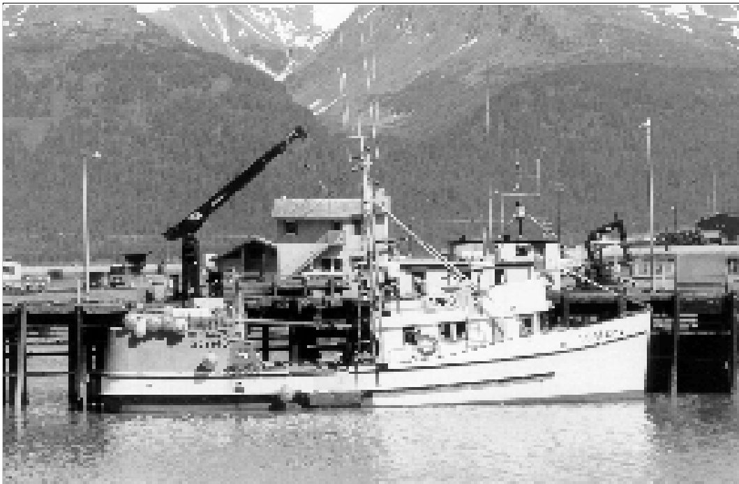
Seine-type vessel Lualda . Note pilothouse forward.
